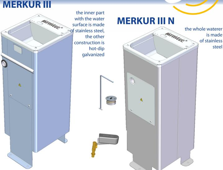
volume 13 l, recommended capacity 15 LSU (1 LSU=500 kg), voltage 230 V, the power consumption 60 W (at 5°C), water flow (at 0,3 MPa) 13 l/min, water supply G 1/2" is in the foot of the waterer, power supply is led to the distribution board in the foot of the waterer, the bottom of the waterer is equipped with a 42 mm diameter plug, IP degree of protection: IP 55
