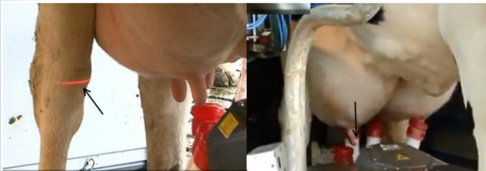
Figure 2. Laser profiles used in the milking robots.
